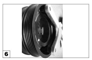
Install the crankshaft pulley, counter-hold pulley with a suitable Holding Tool, such as AST4844, whilst tightening centre bolt, in two stages, 45 Nm. + 90 degrees.
