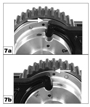
Fit AST4931 VCT Setting Plate on to the VCT Units and check that the timing marks on the **VCT Units and camshaft sprockets** align and are near to the outer edges of the Setting Plate upper arms.
