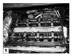
The Ford 1.6 16v. Ti VCT Duratec (Sigma) petrol engine was first introduced in the Ford Focus in 2004. The engine has variable camshaft timing (VCT) on both the inlet and exhaust camshafts.
